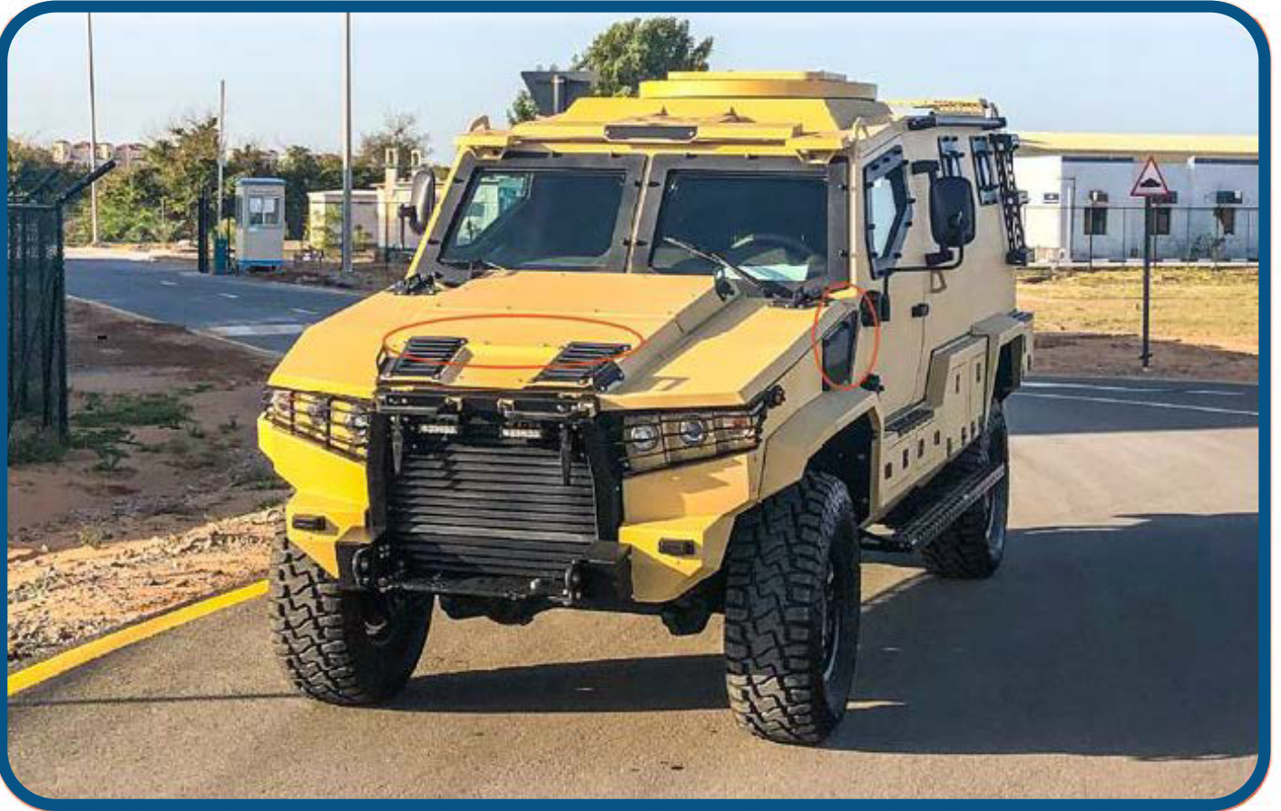
Large Armored Intake Ducts, Fan Assisted Ventilation Ducts
